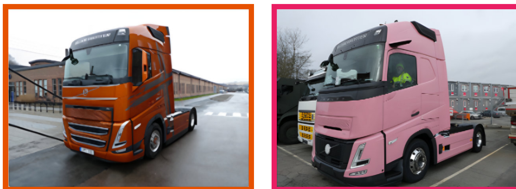
Two Volvo FH trucks with similar drivetrains and trailers: orange with conventional mirrors, pink with CMS.
